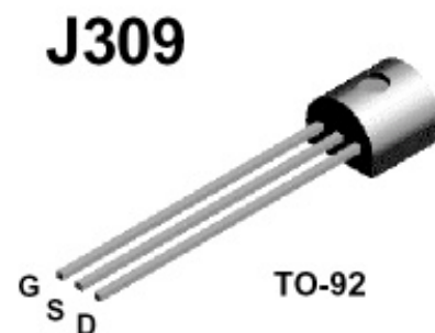
Figure 6: J309 JFET Pin Identification
