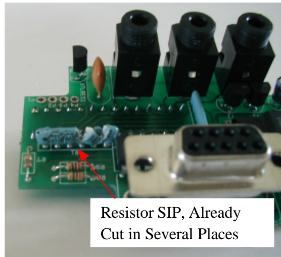
Figure 5: SIP cut for complete removal
